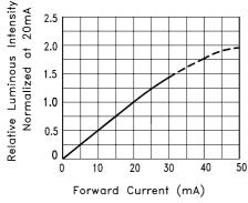
Fig.4 Relative Luminous Intensity vs. Forward Current
